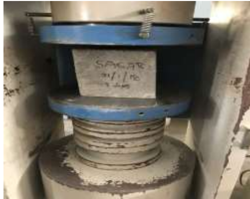
Fig.1. Testing of cube
