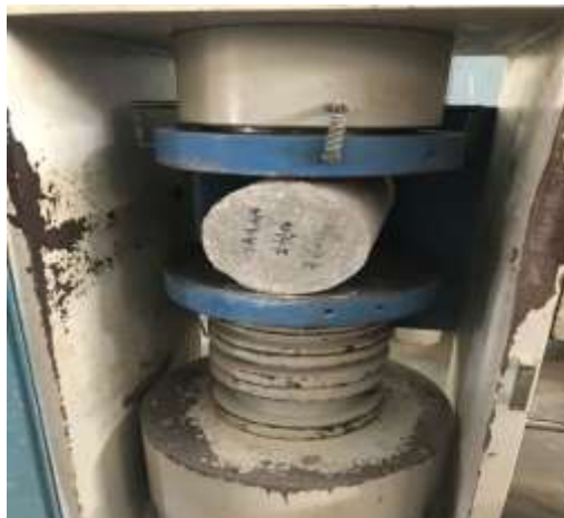
Figure 2. Testing of Cylinder
