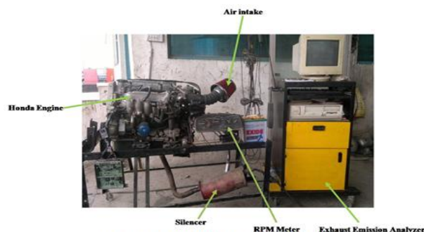
Fig 3 The complete layout of experimental setup.
