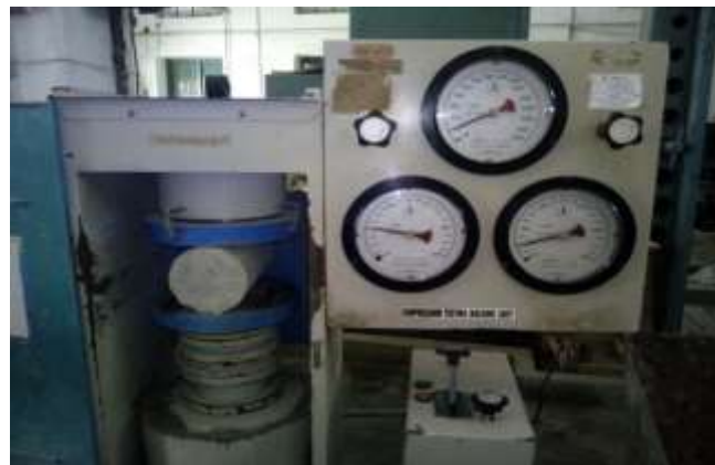
Figure 3. Testing of Cylinder
