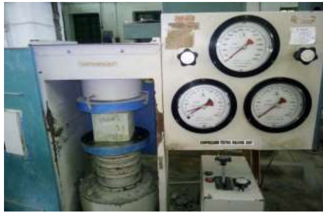
Figure 2. Testing of Cube
