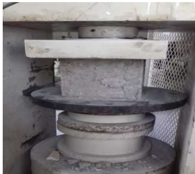
Figure 2: Compressive strength Test
