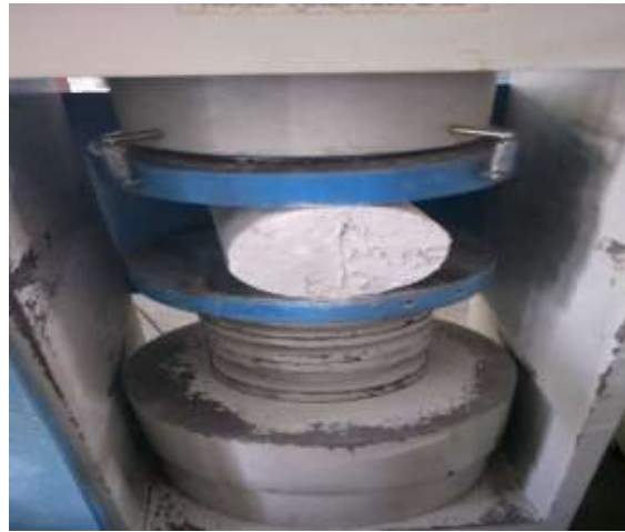
Fig 2. Testing of cylinder
