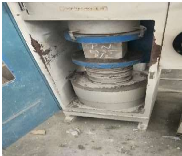
Fig 1. Testing of cube
