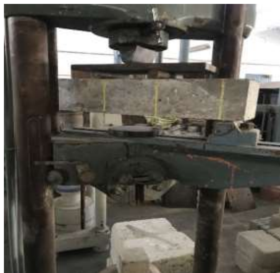
Figure 3. Testing of Prism
