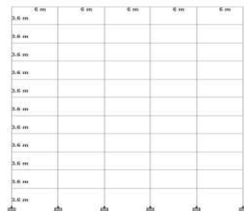
Fig. 4. Elevation of G+10 Building.
