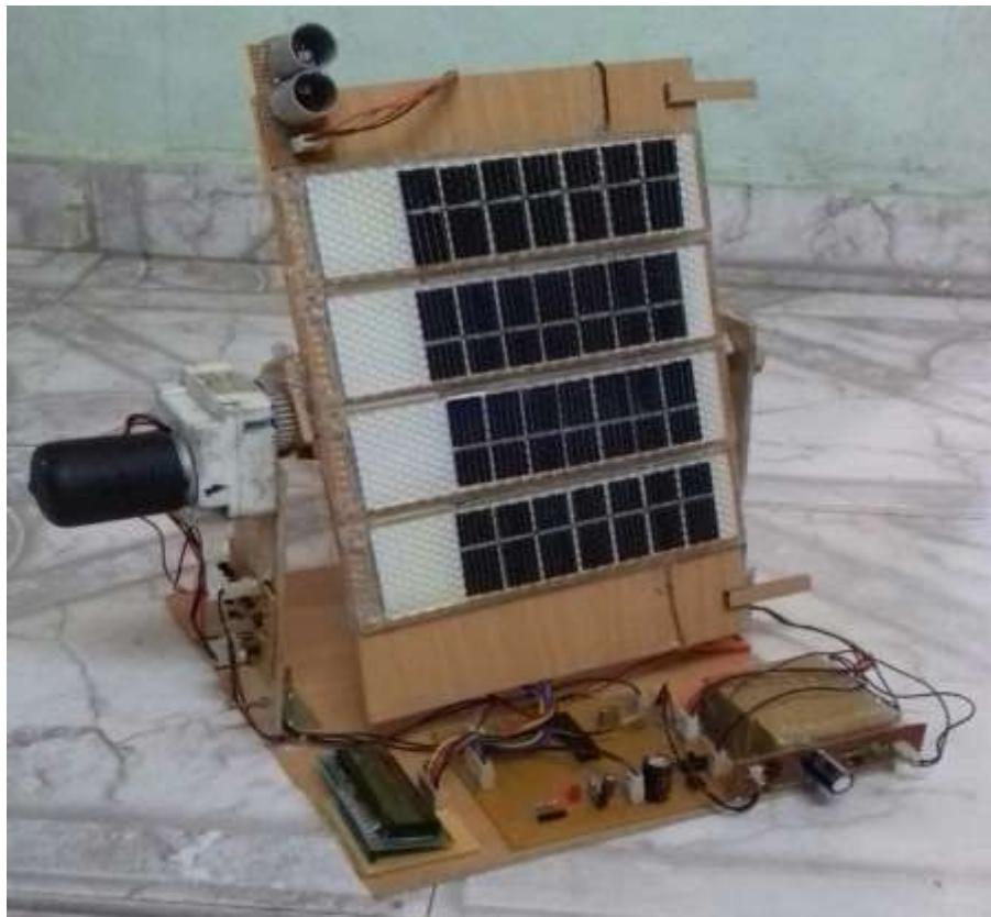
Fig. 3 Experimental setup of solar panel coupled to stepper motor
