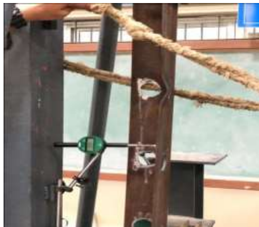
Fig 16 Deflected shape for Three Perforations Angle member
