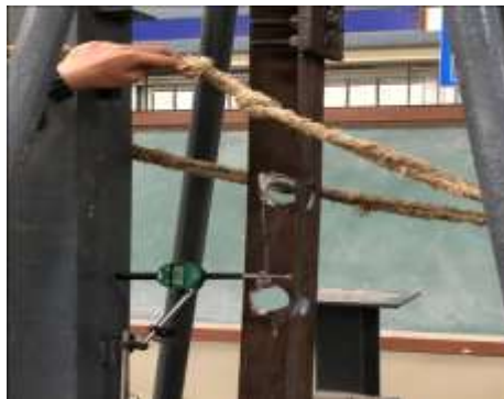
Fig 15 Deflected shape for Two Perforations Angle member
