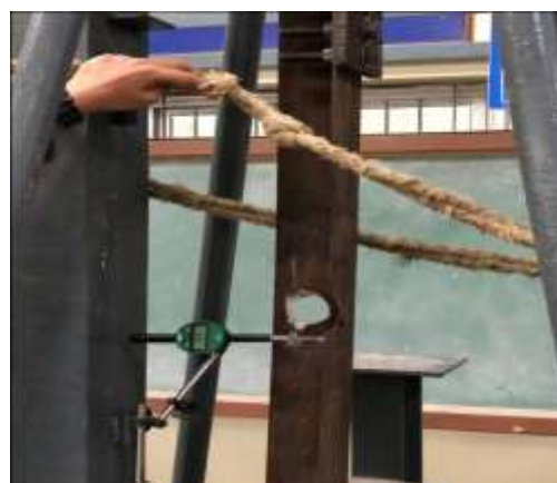
Fig 14 Deflected shape for Single Perforations Angle member
