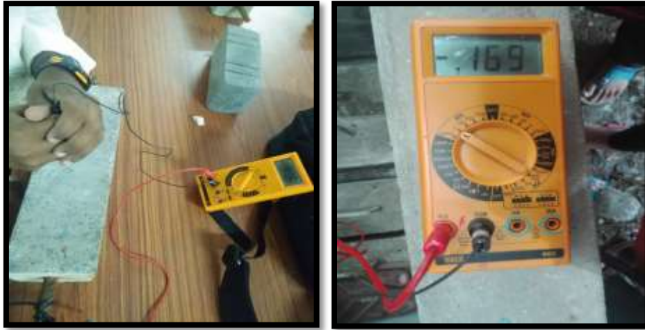
Fig 7: testing of specimen by OCP method
