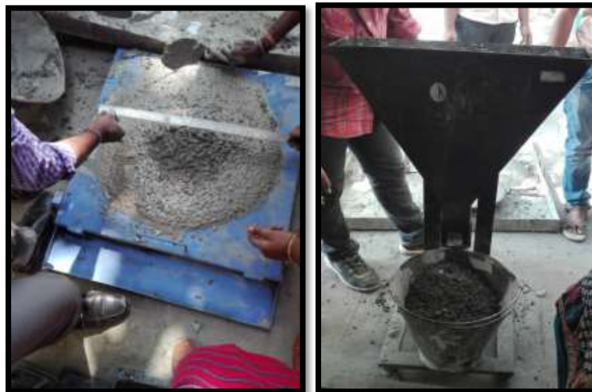
Fig3: slump cone and V-funnel tests
