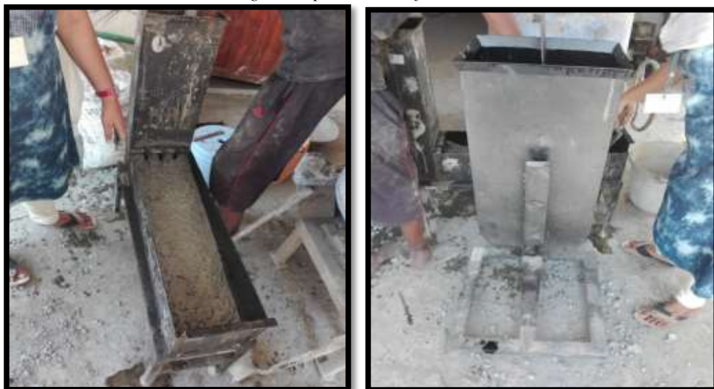
Fig 4: L-box and U-box tests
