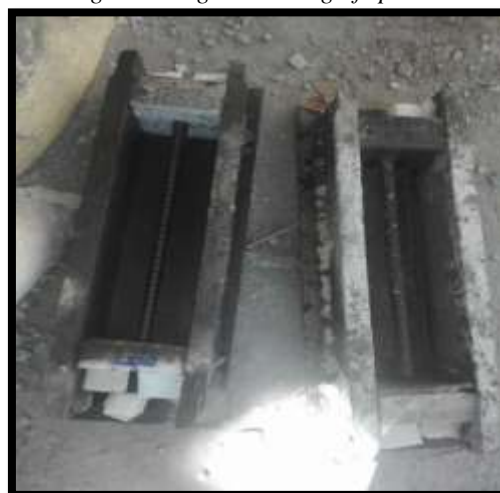
Fig 2: Formwork of specimen for corrosion test
