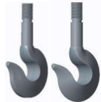
Figure 5.2: 3D Models of Triangular and Trapezoidal Cross-section Crane hook
