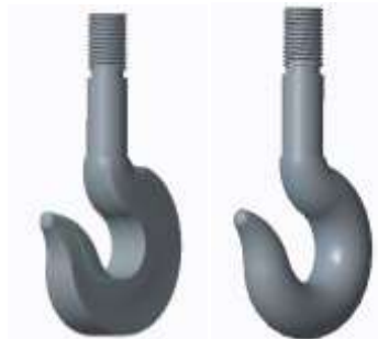
Figure 5.1: 3D Model of Rectangular and Circular Cross-sections Crane hook
