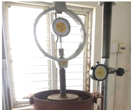
Fig.2 Proving Ring Attachment.
