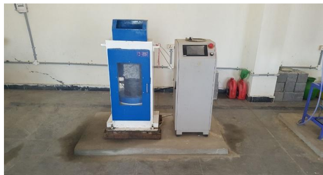
Figure 6.3: Compression testing of Cube Specimen
