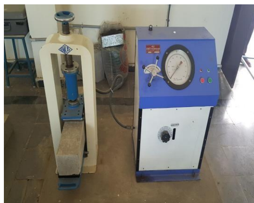
Figure 6.5: Flexural Testing of Beam Specimen
