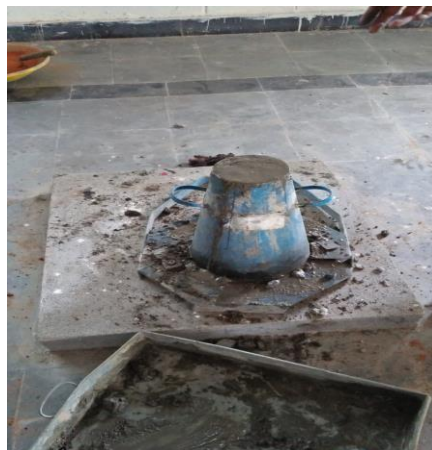
Figure6.1: Concrete Slump Test Procedure
