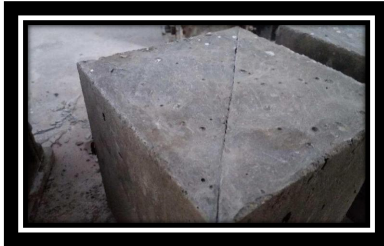
Fig 3. 91days healing concrete
