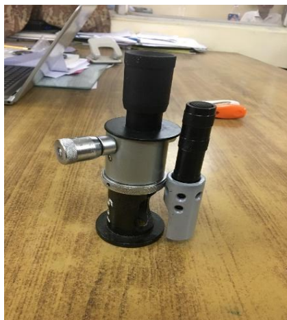
Figure 6: Micrometer used for measuring width of crack
