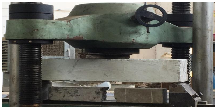
Figure 7: Analyzing Beam Strength on Universal Testing Machine
