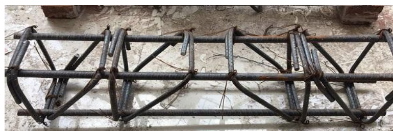
Figure 4: Beam Reinforcement with combination of Stirrups
