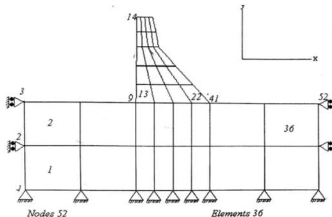
Fig.4 Finite element division of Koyna dam
