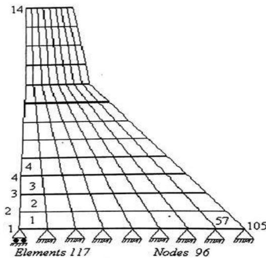
Fig.7 Finite element division of Koyna dam
