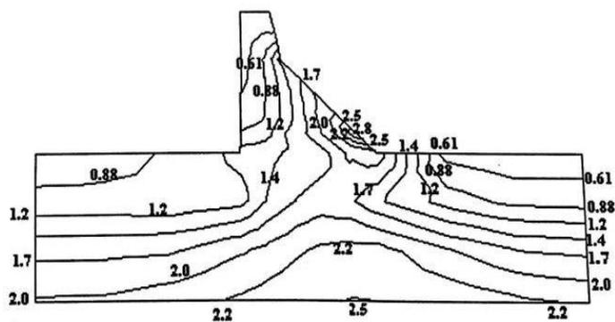
Fig.10 Vertical normal stress contours for case 2 in N/sq mm
