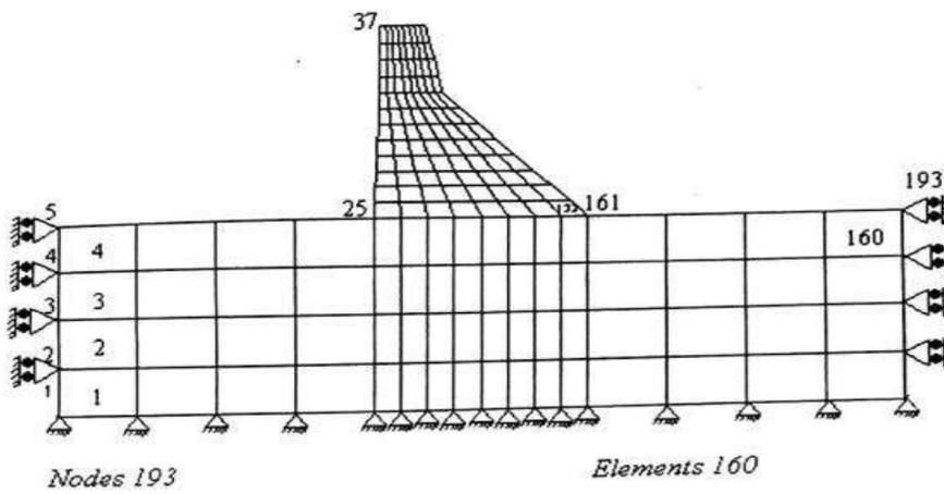
Fig.6 Finite element division of Koyna dam
