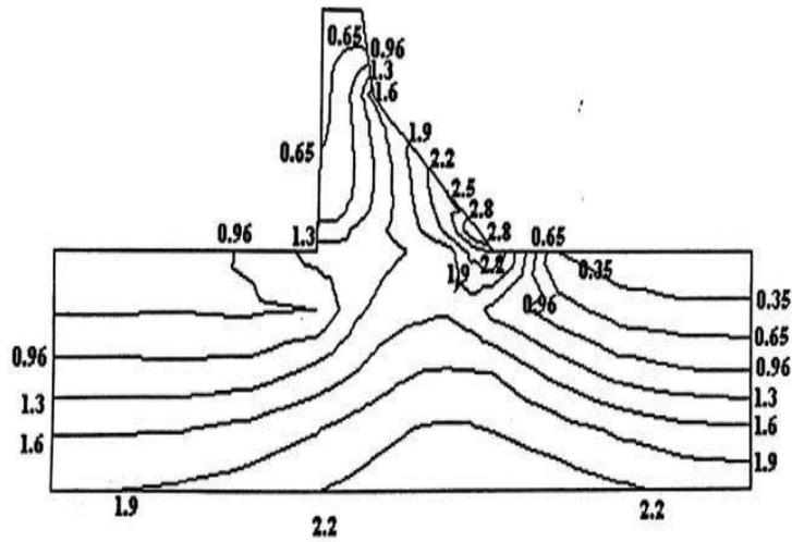
Fig.11 Vertical normal stress contours for case 3 in N/sq mm
