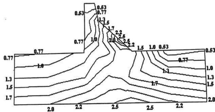
Fig.9 Vertical normal stress contours for case 1 in N/sq mm
