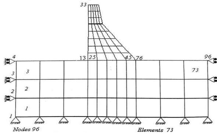
Fig.5 Finite element division of Koyna dam
