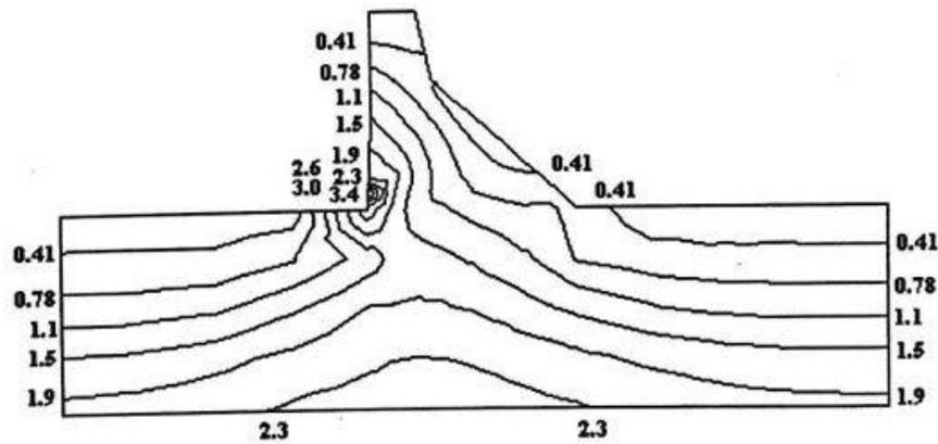
Fig.14 Vertical normal stress contours for case 6 in N/sq mm
