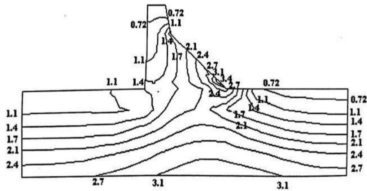
Fig.12 Vertical normal stress contours for case 4 in N/sq mm
