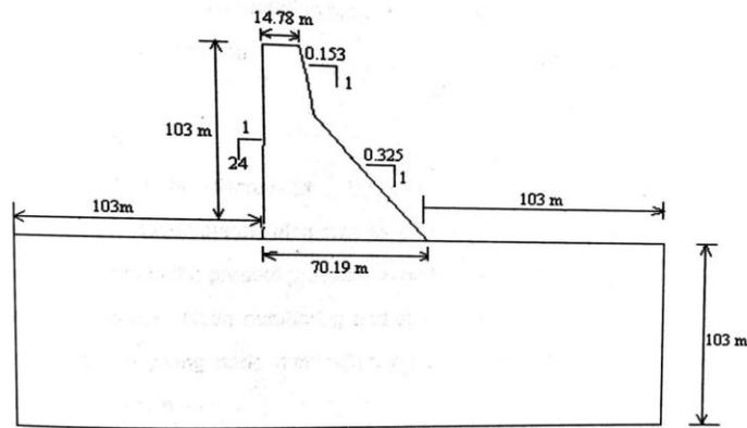
Fig. 3 Cross section of the dam along with the foundation rock
