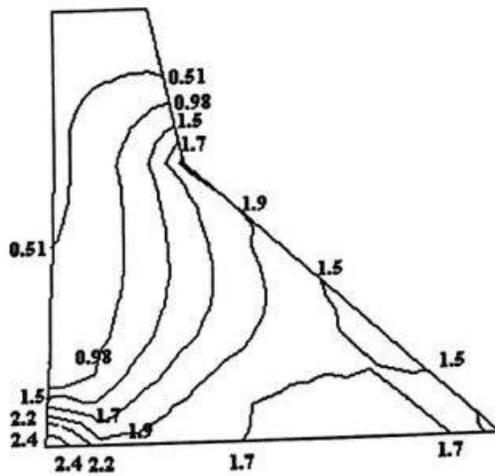
Fig.13 Vertical normal stress contours for case 5 in N/sq mm
