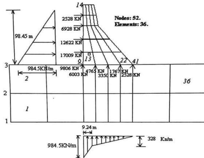
Fig.8 Distribution of water pressure on u/s side and uplift pressure at the foundation interface of a dam.
