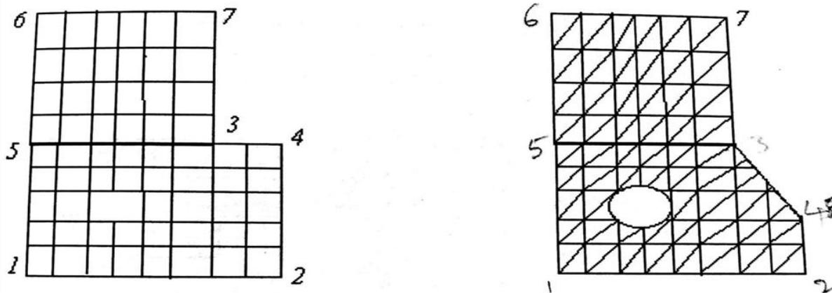
Fig.1 Mapping from (I, J) to (x, y) space
