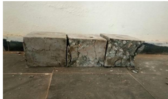
Fig 10: after testing in CTM the cubes were like this
