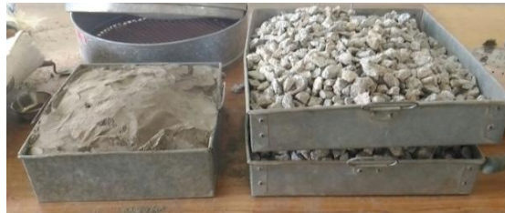
Fig 4: batching of concrete ingredients
