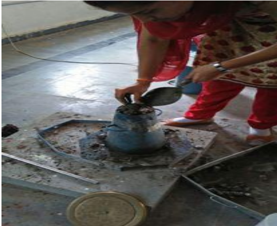
Fig 6: slump cone with concrete Casting
