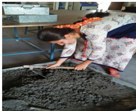
Fig 5: Hand mixing of concrete
