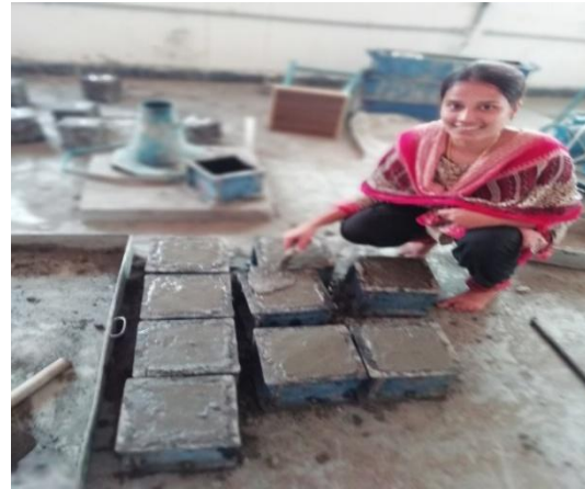
Fig 7: casting of concrete cubes Curing
