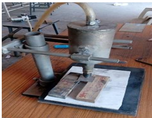
Fig. 1: Machining of Nimonic alloy 75 Using AJM
