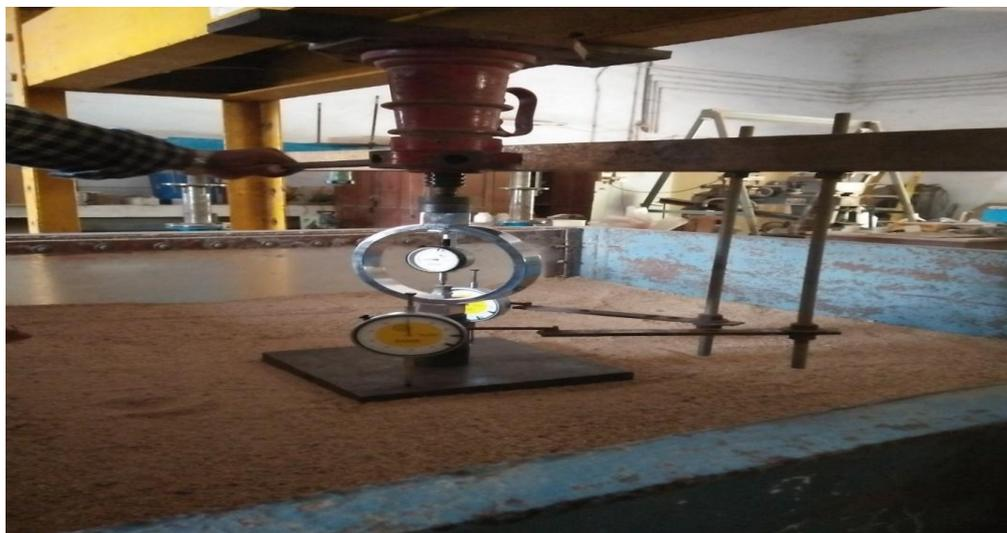
*Fig.3 Arrangement of vertical loading of cyclic plate and dial gauges*
