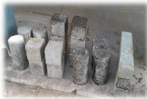
Figure 1: Shows the casted Cured specimens
