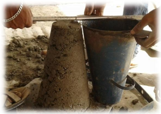
Figure 2: Shows Slump cone test
