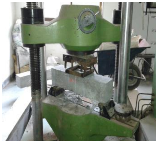
Fig. 5. Flexural strength test setup
