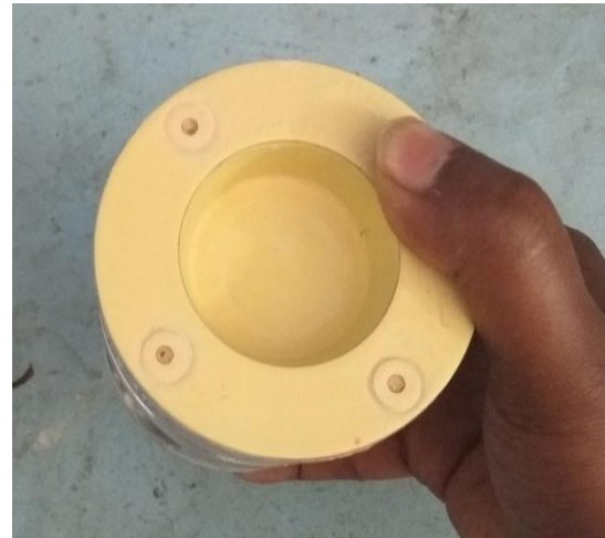
Figure 4: Yttrium Oxide Coated Piston
