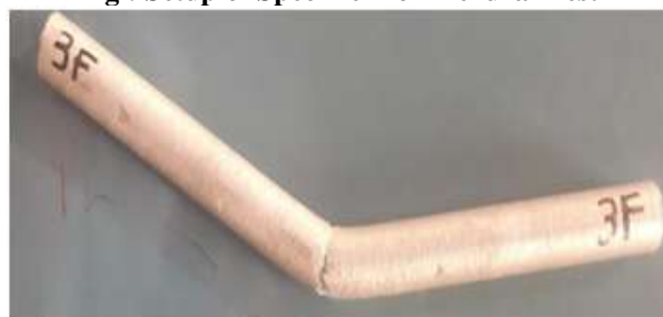
Fig : Specimen after Flexural Test
