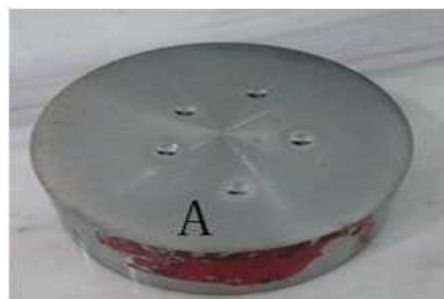
Fig:Specimen after Hardness Test
