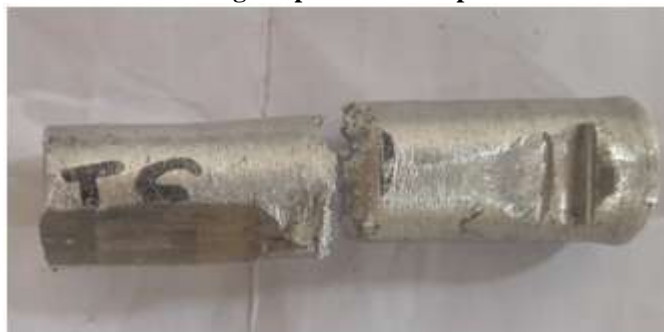
Fig :Specimen after Impact Test
