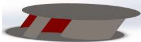
Figure: Four blades Savonius rotor design
