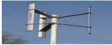
Figure : H-Darrieus rotor
