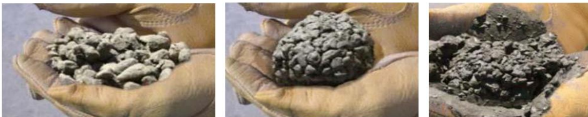
Fig: Concretewith a. Too little Water, b. Appropriate Amount of Water, c. Too much Water
