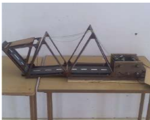
Figure-01-folding bridge model of descending equilateral triangle
