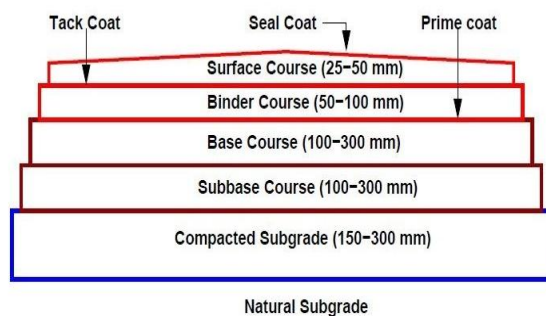
Typical cross section of a flexible pavement
