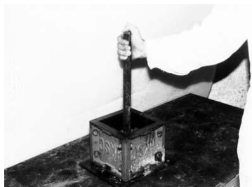
Compacting the concrete in the cube mould
