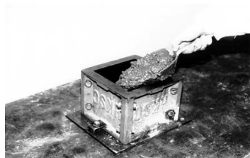
Filling the mould (for 150 mm cube 3 equal layers)
