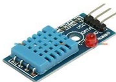
Fig.3.DHT11SENSOR(combination of temprature and humiditi sensor)
