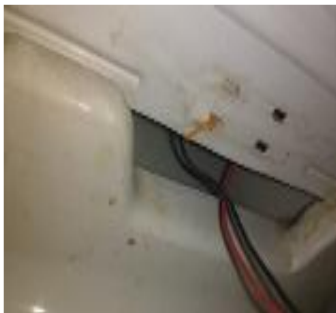
Fig 2 Peltier module at the evaporator
