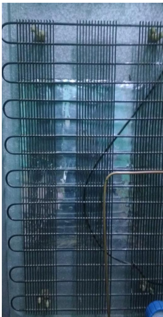
Fig 3 pcm encapsulation at the condenser
