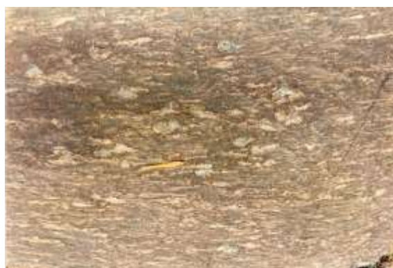
Fig. 10. Metapelite showing dull white to cream coloured porphyroblasts of sillimanite oriented parallel to the foliation (0.5 km SW of Duntur).
