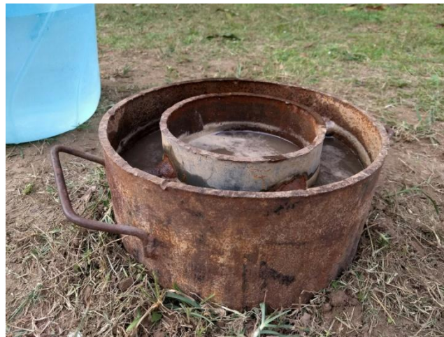
Figure 2 Measurement of depth during the field investigation using Double Ring Infiltrometer
