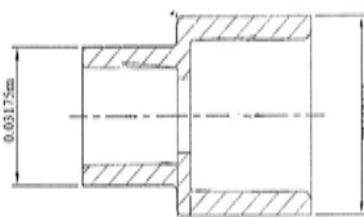
Figure 6: Dimensions of Reducer
