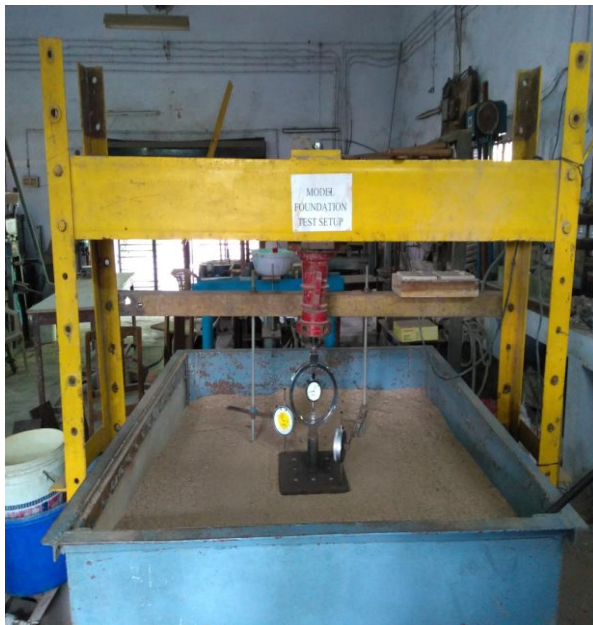
Fig 4 Model foundation test set and loading arrangement
