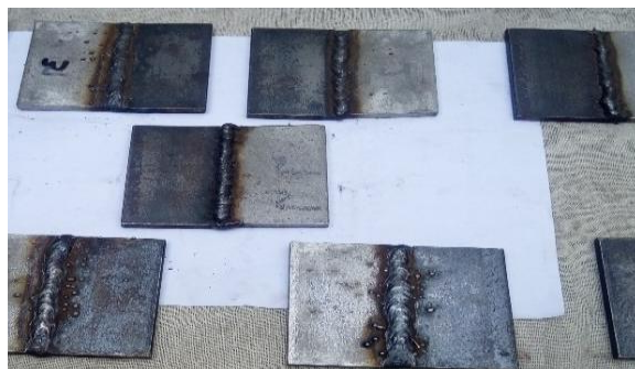
Fig. 3 Welded specimen of SS 202 and AISI 1018
