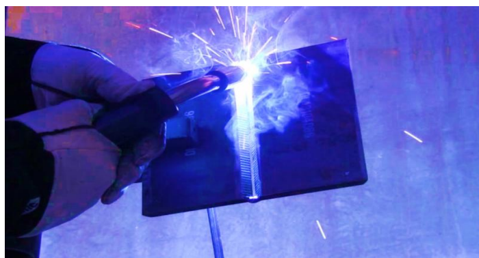
Fig. 2 GMAW of SS 202 and AISI 1018
