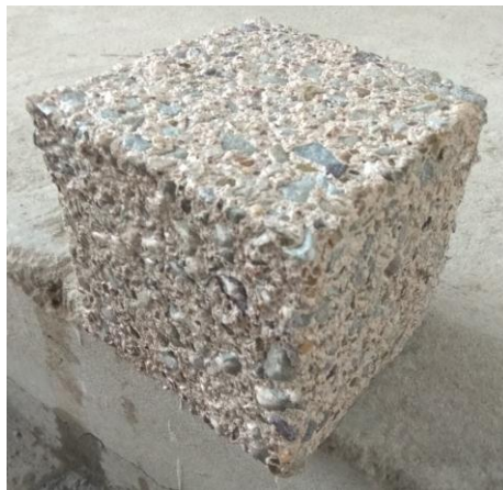
Fig 2 Specimen after being immersed in acidic solution for 56 days
