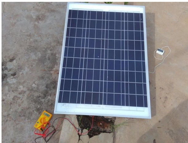
Fig. 75w PV panel and aluminum tray with PCM
