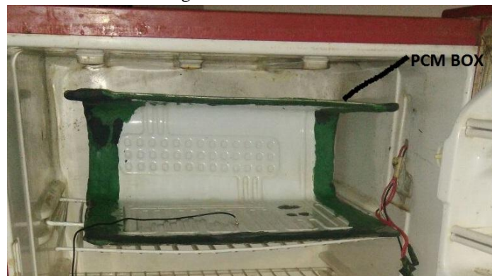
Fig 2. Fabricated PCM box fitted around the cabin
