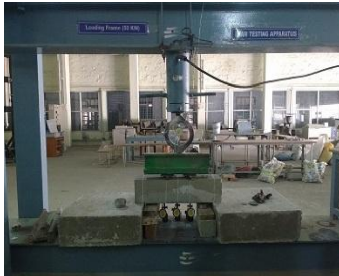
Figure-4. Experimental set up for beam in loading frame
