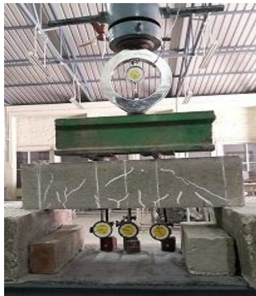
Figure-5. Flexural Test on SCGC beam
