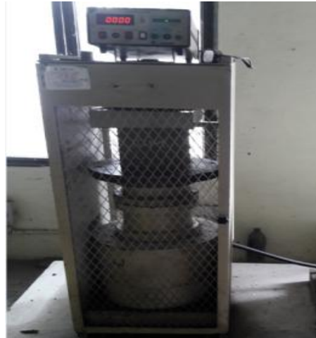
Figure-2.Compressive test on SCGC cube
