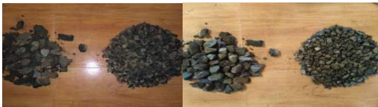
Figure 4.1 RAP materials before and after extraction of asphalt content.
