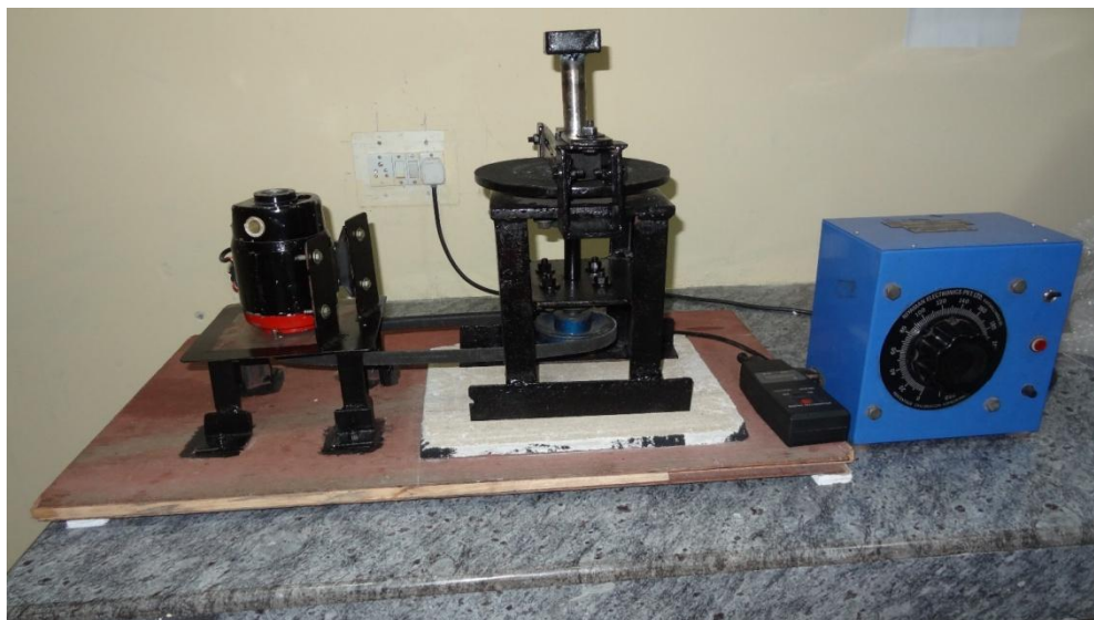
Fig.2 Actual photograph of the two-body abrasion setup.
