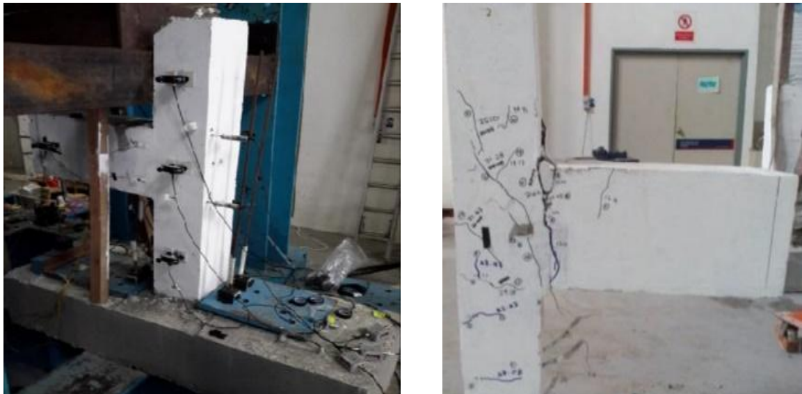
Figure 1 RC beam column junction test setup and mapping of crack produced [5]
