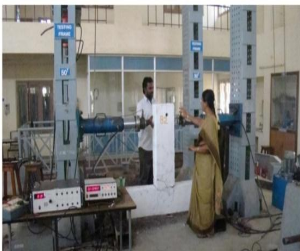
Figure 4 Test setup and crack pattern of RCC beam column junction [13]
