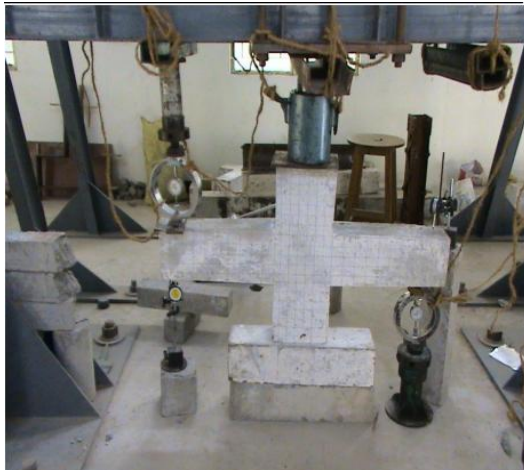
Figure 3 RC beam column junction test setup and load vs deflection behaviour [9]
