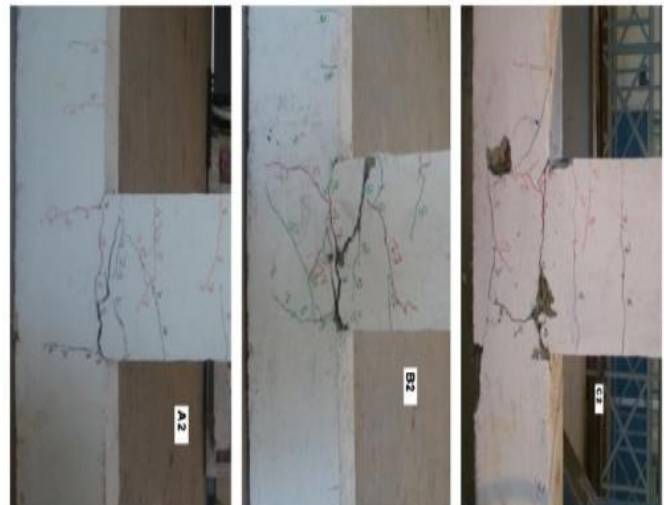
Figure 4 Test setup and crack pattern of RCC beam column junction [13]
