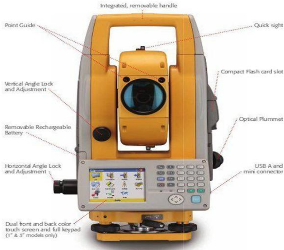
Fig 1 : Total station details [1]
