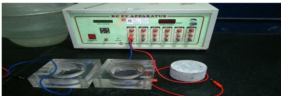
Fig. 3 Rapid Chloride Permeability Test
