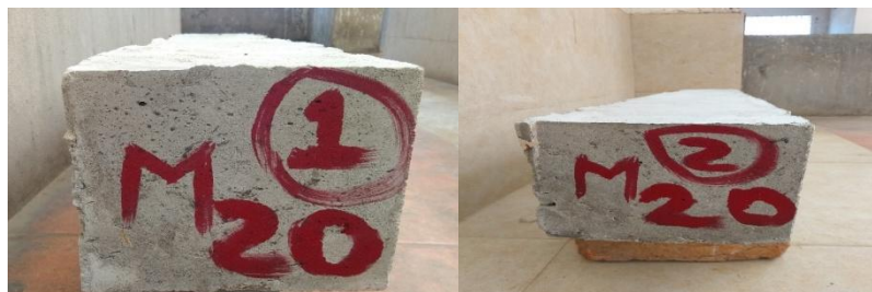
Fig 1 RCC beam with M20 grade (1) and GFRP beam with M20 grade (2)
