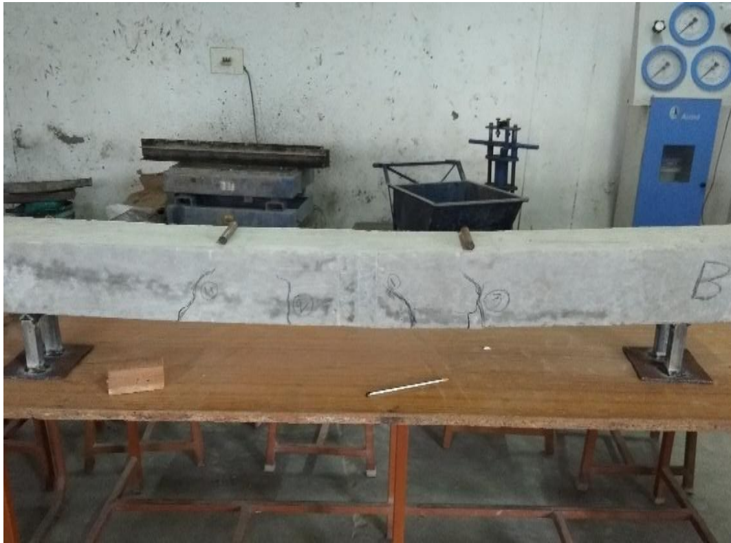
Fig 9 Crack pattern for beam specimens
