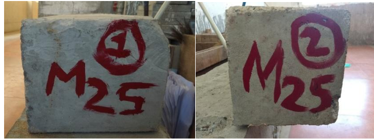
Fig 2 RCC beam with M25 grade (1) and GFRP beam with M25 grade (2)
