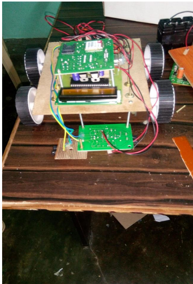
LPC2148 interfacing with robot peripherals
