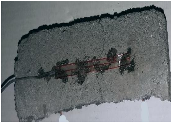
Figure 3 a) Cracked specimen with strain gauge sensor b) TMR 7200 which shows strain gauge sensor data with data logger
