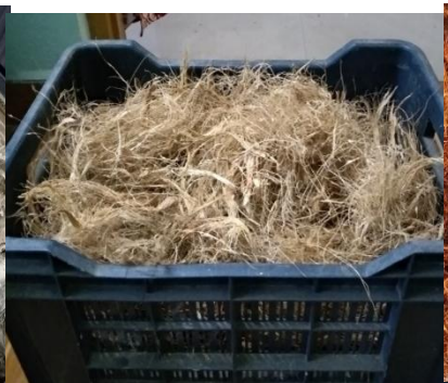
Fig:2 (b) Coir separated by pounding
