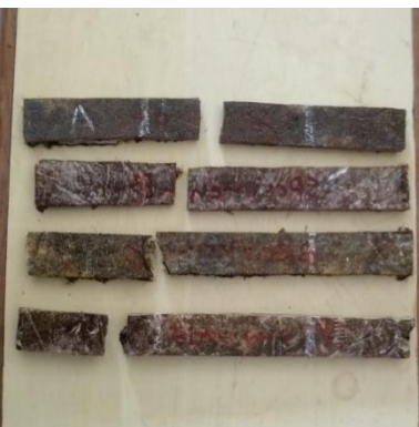
Fig: 5(c) Specimens after Tensile Testing
