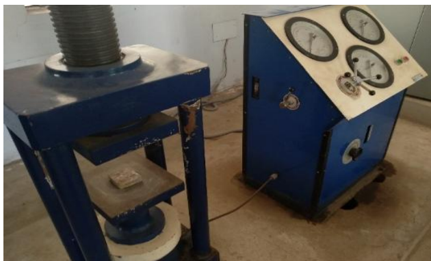
Fig 6: Specimen loaded in Compression Testing Machine
