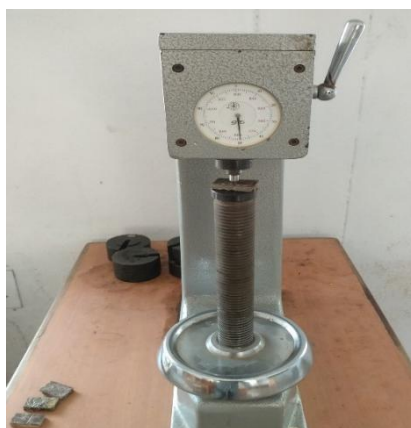
Fig 7: Specimen Loaded for Brinells Hardness Test
