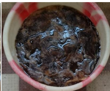
Fig: 4 (b) Fibre in 5%NaOH Solution
