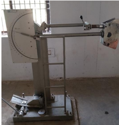
Fig 8: Specimen loaded for Impact Test
