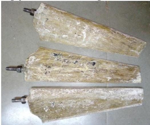
Fig.1: Flax Fibres with Polyester Blades
