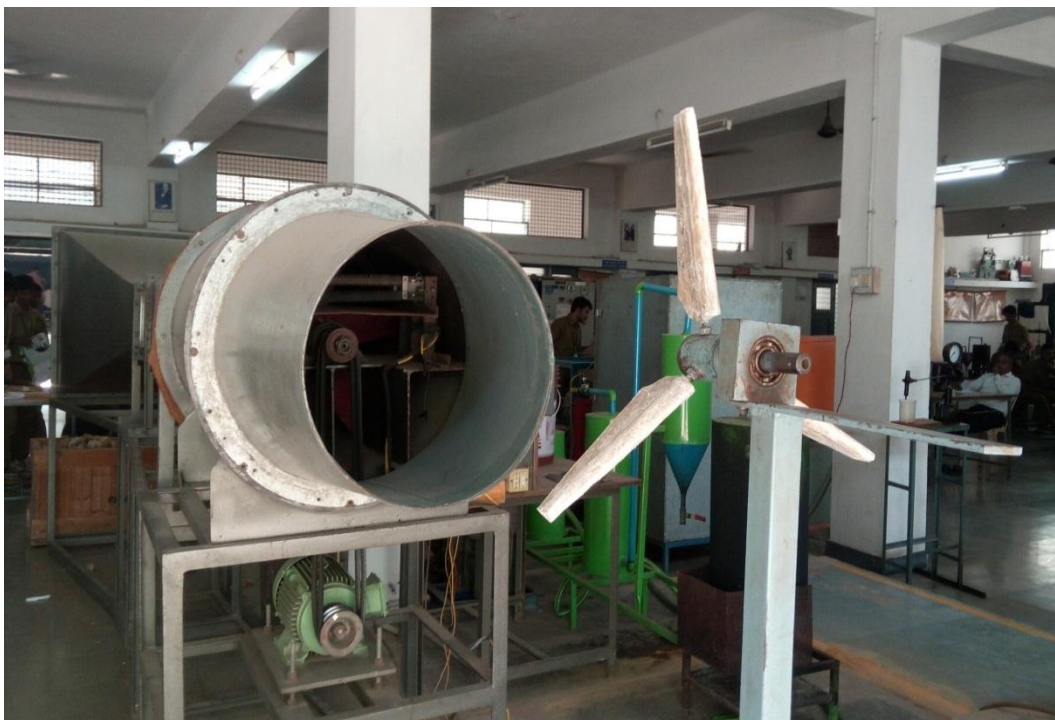
Fig.3 Wind turbine made of flax fiber blades near wind tunnel
