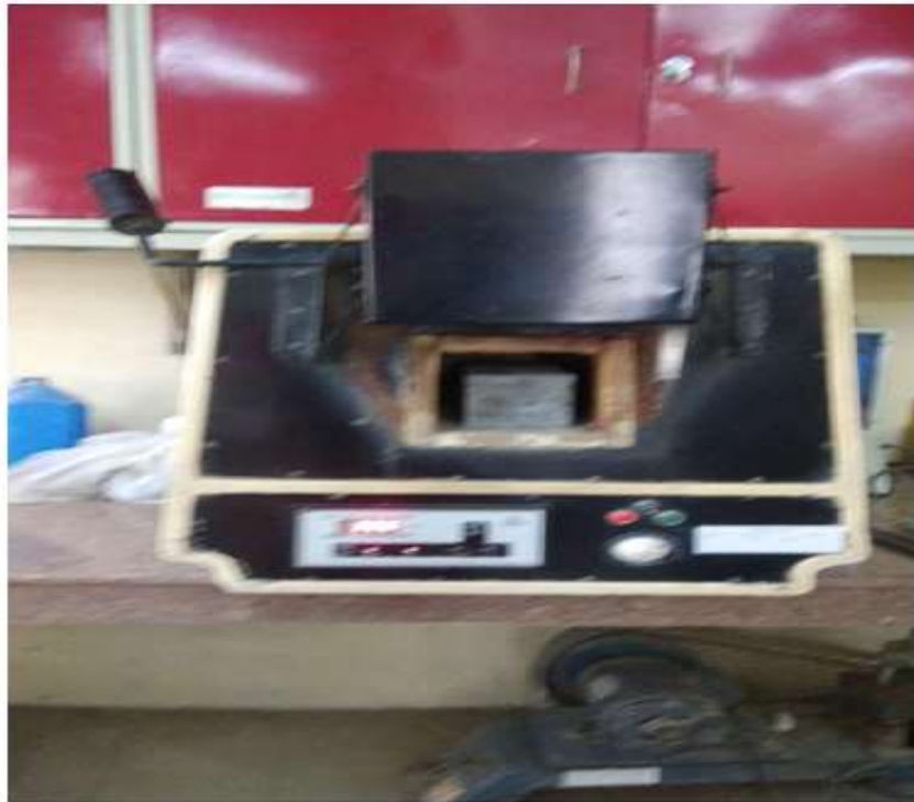
Figure 6.1 furnace used to heat the specimens
