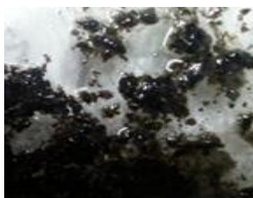
Fig. 9. Flocculation of particles when graphene oxide is incorporated into cement [25]
